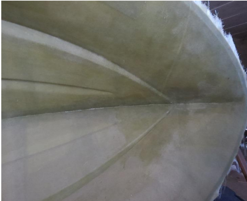
9 layer hand laid hull seen in the mold.
